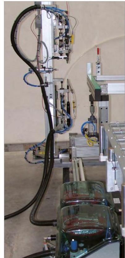
Example of MCA tightening module for shutters field: assembly from the top towards the bottom and from bottom towards the top
