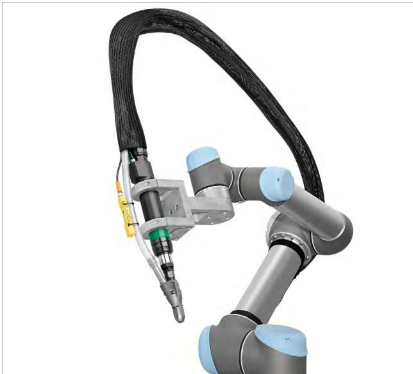
Example of MCA tightening module with collaborative robot
