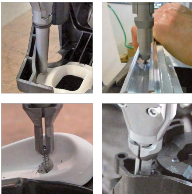
Examples of special heads with friction jaws to access to deep tightening points, behind shoulders or for entering very narrow holes.
