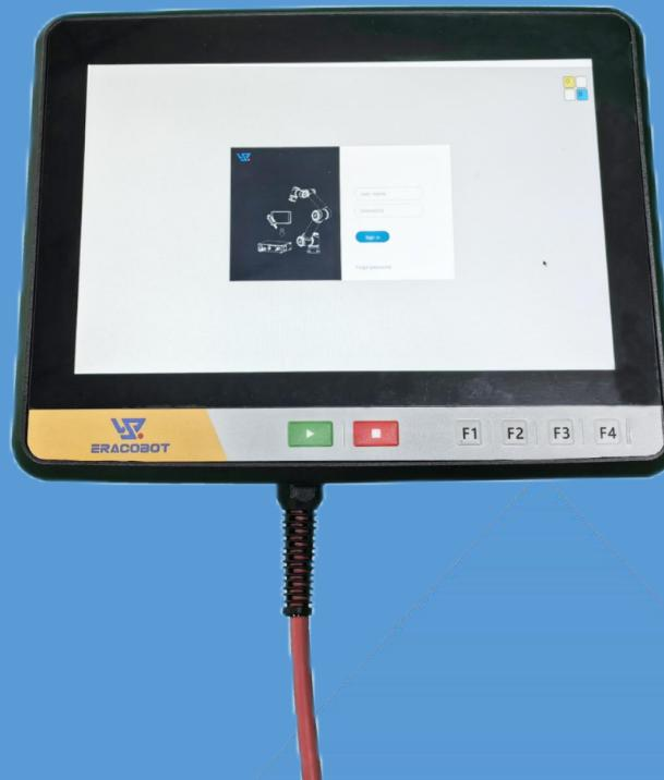
The teach pendant, computer, tablet or mobile phone is connected to the WebAPP system to realize the operation of the collaborative robot.
